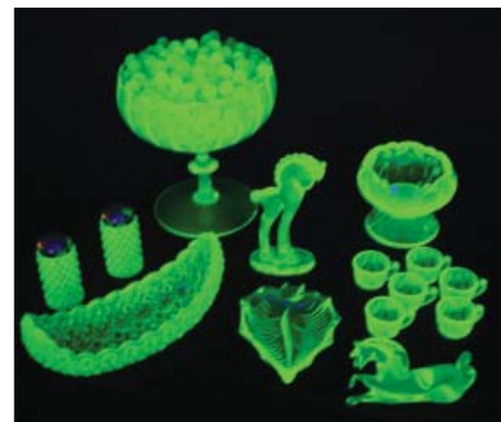
Fig. 6. The uranium content of the Vaseline glass causes it to fluoresce under ultraviolet light.
