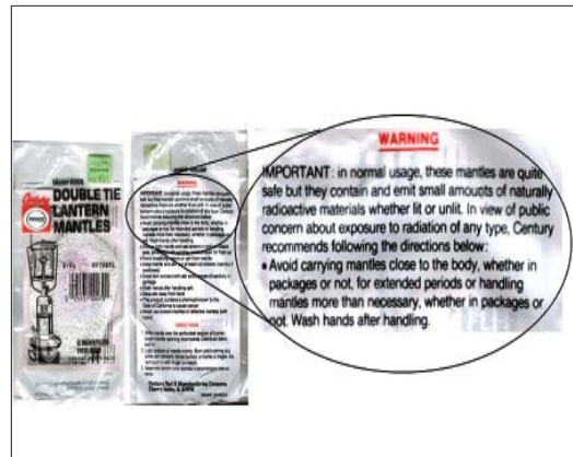
Fig. 3. Radioactive lantern mantles containing thorium nitrate.
